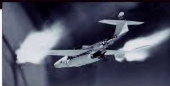
Above: As a dedicated bomber destroyer, the original weapons fit for the F-89 was 104 unguided rockets housed in wing-tip pods. Good stability was needed to cope with the buffet created on launching.
